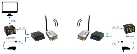
DTC + amplifier radios and 1x operation
