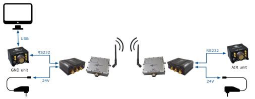
Microhard + amplifier radios and Autopilot 1x operation
